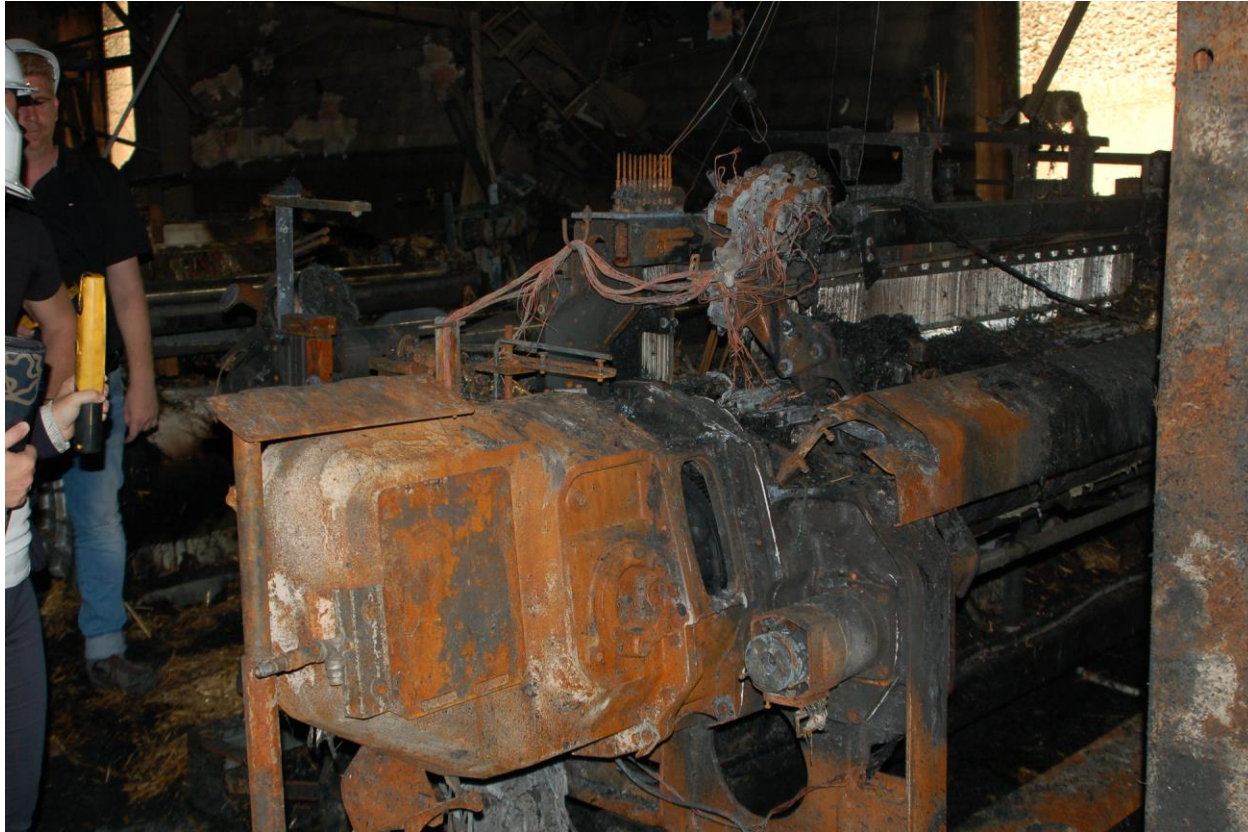
Machinery – A loom after a fire loss. The loom engine was the fire origin
