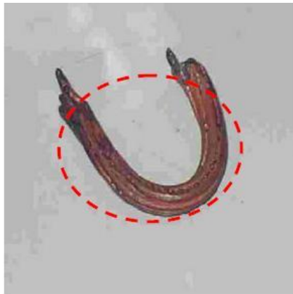
Short circuit with cable fusion
