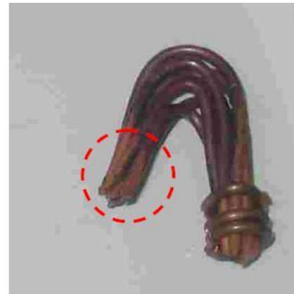
Short circuit with cable fusion
